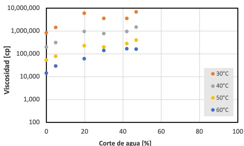
a. System "A": stable emulsions were generated with water cuts of up to 50%, the surfactant reduced the viscosity of the emulsions to values lower than that of pure oil and this effect increased with the upsurge in the water cut.
